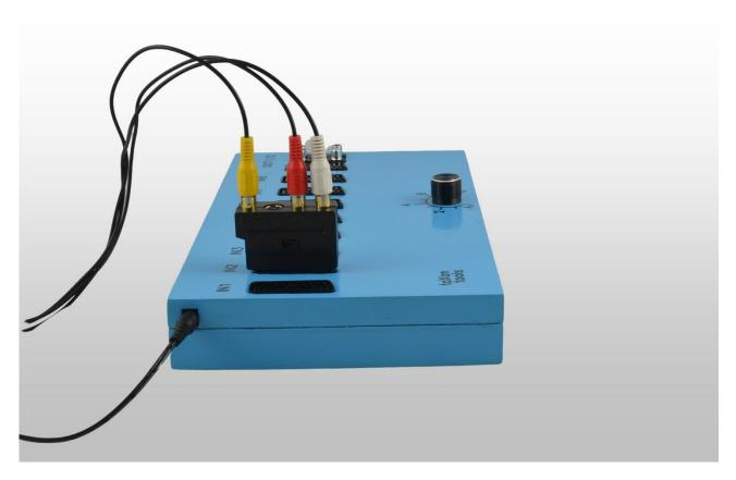
If you want to connect devices with RCA connectors, use either the Taxon Tools adapter or an equivalent adapter to convert RCA to Scart. Connect the corresponding color of the RCA cable to the same color of the adapter.
