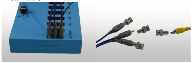
A Sony PVM monitor can be connected directly. All you need is 4 RCA-to-BNC adapters (RCA: female, BNC: male) on the monitor side. Connect the video output (yellow) and the three colors (red, green, blue) to the corresponding inputs of the Sony PVM monitor.
